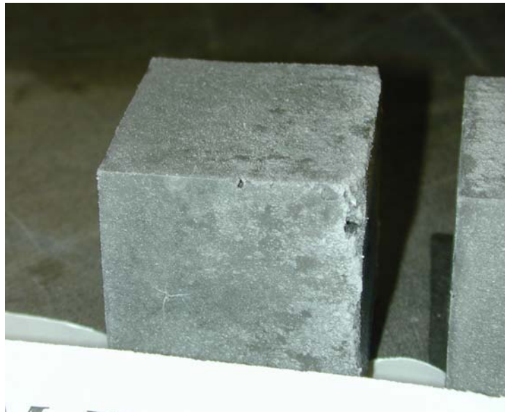
Figure 8 Cube specimen after 1 month in \text{MgHPO}_4 .
