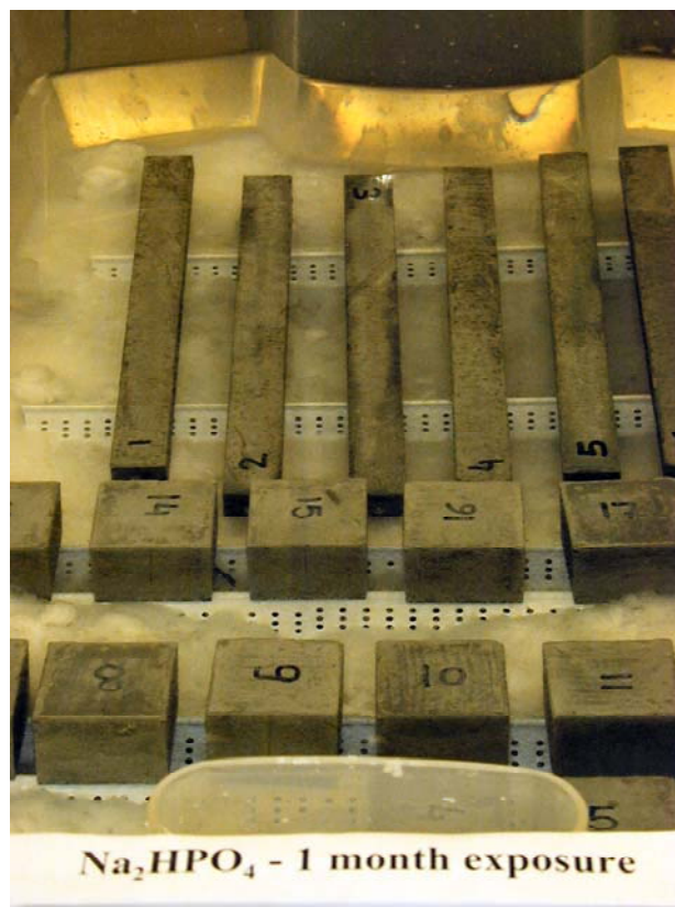
Figure 6 Exposure testing in saturated brines in which PVC corner braces are used to suspend cubes and prisms above the excess solids (visible).
