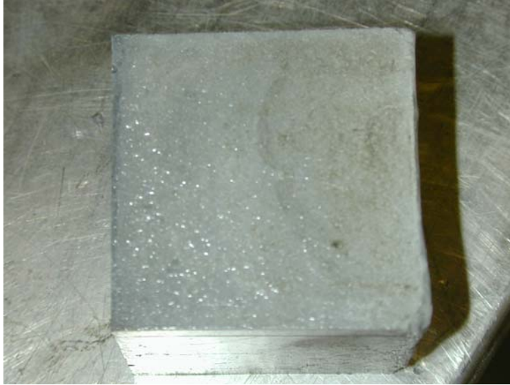
Figure 9 Cube specimen after 1 month in \text{Na}_2\text{HPO}_4 .
