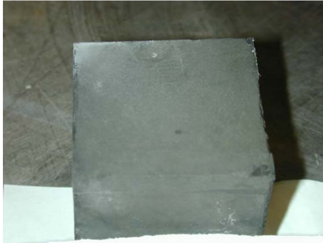
Figure 6 Cube specimen after 1 month in \text{Ca}(\text{OH})_2
