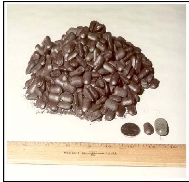
Fig. 11. DUAGG briquettes produced at Starmet.
